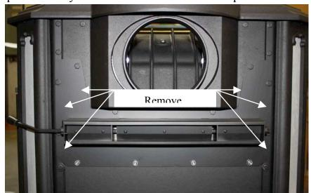
be used to remove the bolts at either end of the damper assembly.
