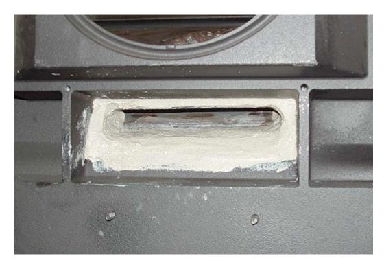
11. Through the loading door, apply cement along the bottom of the secondary fireback.
